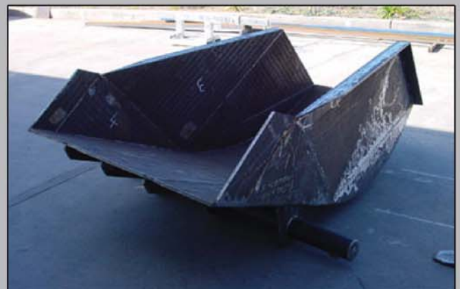
50n8 Head End Clamshell fabricated from Duaplate
