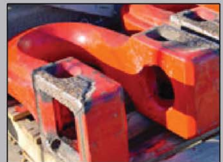
Tungsten Chip Hard facing to Drag Shackle
